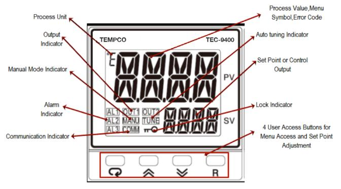
TEC-9400 Front Panel Keys and Display
