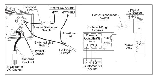
Figure 1. Application Wiring Example (single-zone shown)
