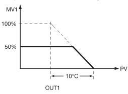
Figure 4.5 Power Limit Function
