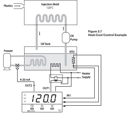
PID heat-cool is used for the above example.
