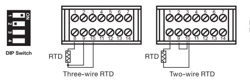
Figure 2.6 RTD Input Wiring
