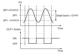
Setup ON-OFF: OUT1= <u>r E <u>r</u></u> PB1=0 Adjust: SP1, O1HY, TIME(if enabled)
