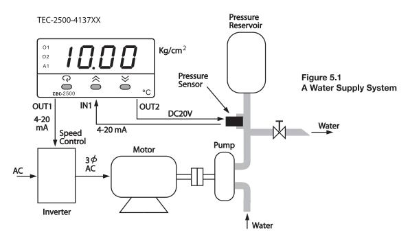
The water pressure in this example must be controlled at 10Kg/cm<sup>2</sup>. To achieve this, the following devices are used for this example:
