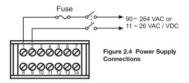
This equipment is designed for installation in an enclosure which provides adequate protection against electrical shock. The enclosure must be connected to earth ground.
