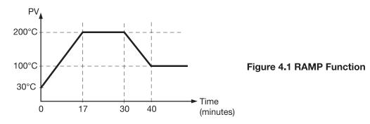
**Note:** When the ramp function is used, the display will show the current process value. However, it will revert to show the set point value as soon as the up or down key is pressed for adjustment. Setting RAMP to zero means no ramp function at all.
