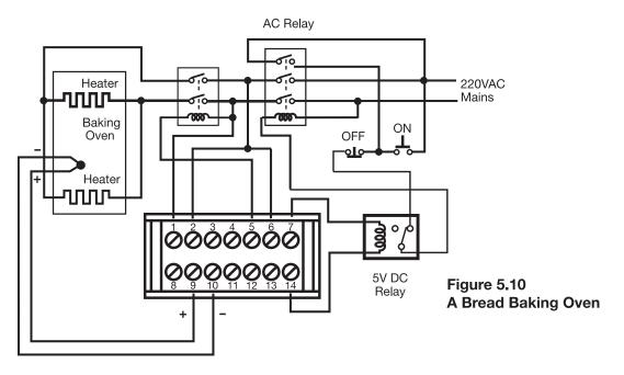
Push the ON switch to start a batch. The temperature will rise with a ramp rate determined by the RAMP value. The bread is baked with the set point temperature for a predetermined amount of time which is set in the TIME value, and then the power is shut off. The temperature profile is shown in the following figure.
