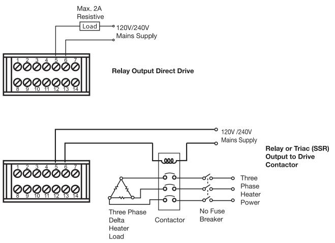
Figure 2.14 Output 1 Wiring
