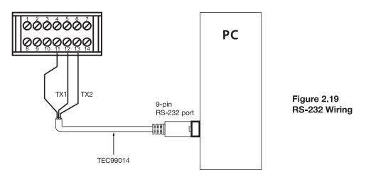
Note: If the TEC-2500 is configured for RS-232 communication, the input 2 and EI (Event Input) are disconnected internally. The unit can no longer perform event input functions (EIFN) or input 2 functions.
