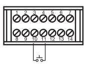
Figure 2.13 Event Input Wiring
