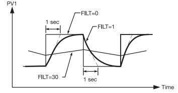
Figure 4.7 Filter Characteristics
