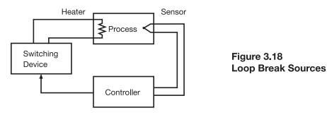
Loop Break Sources: Sensor, Controller, Heater, Switching Device
