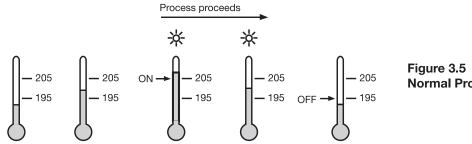
Figure 3.5 Normal Process Alarm
