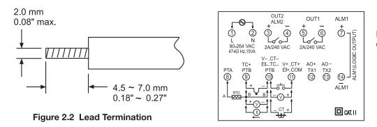
Figure 2.3 Rear Terminal Connection Diagram
