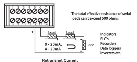
Figure 2.22 Analog Retransmission Wiring
