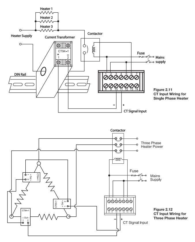
Make sure that the total 3-phase current does not exceed 100A rms.
