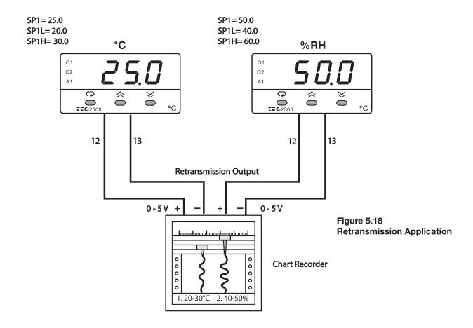
SP1L and SP1H are used to limit the adjustment range of the set point.
