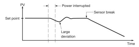
Since the hardware and software need time to be initialized, the control is abnormal as the power is recovered and results in a large disturbance to the process. During the sensor breaks, the process loses power.
