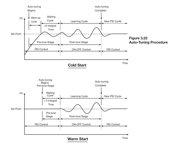
If auto-tuning begins near the set point (warm start), the unit skips the warm-up cycle and enters the waiting cycle. Afterward, the procedures are the same as described for cold start.
