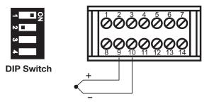
If the length of the thermocouple plus the extension wire is too long, it may affect the temperature measurement. A 400 ohms K type or a 500 ohms J type thermocouple lead resistance will produce approximately 1°C temperature error.
