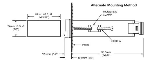
Figure 2.1 Mounting Dimensions
