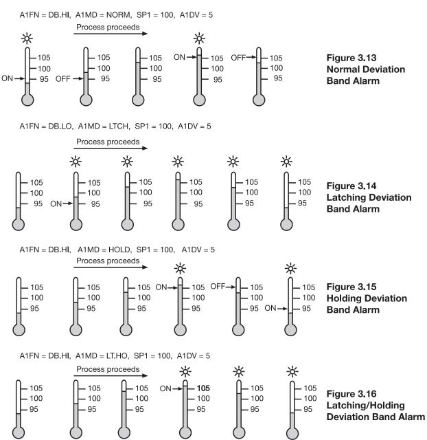
2 types of deviation band alarms: DB.HI, DB.LO Deviation band alarm 1: Setup: A1FN, A1MD Adjust: SP1, A1DV Trigger level=SP1±A1DV Deviation band alarm 2: Setup: OUT2, A2FN, A2MD Adjust: SP1, A2DV Trigger level=SP1±A2DV
