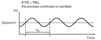
Figure 3.24 **Critical Steady State**
