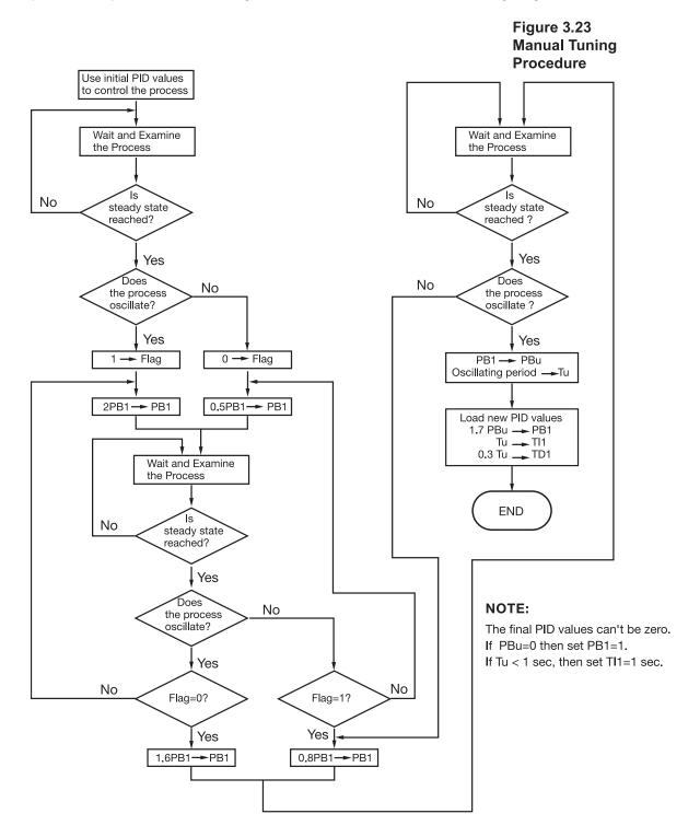
The above procedure may take a long time before reaching a new steady state since the P band was changed. This is particularly true for a slow process. As a result, the above manual tuning procedures will take from minutes to hours to obtain optimal PID values.
