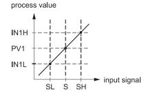
Figure 3.1 Conversion Curve for Linear Type Process Value
