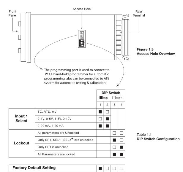
The programming port is used for off-line automatic setup and testing procedures only. Do not attempt to make any connection to these pins when the unit is being used for normal control purposes.
