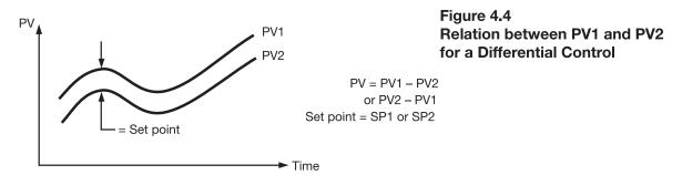
The PV display will indicate PV1-PV2 value if P1-2 is chosen for PVMD, or PV2-PV1 value if P2-1 is chosen for PVMD. If you need PV1 or PV2 to be displayed instead of PV, you can use the display mode to select PV1 or PV2 to be viewed. See section 3-24.
