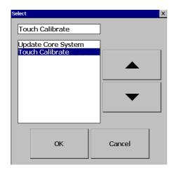
This is used to calibrate the touch screen. A "+" symbol appears in the center of the LCD screen. Carefully press and briefly hold a stylus or finger on the center of the target. Repeat this procedure as the target moves around the screen. Just touch the screen to complete the screen calibration. This procedure helps to locate pointer via touch screen and properly select the objects during operation of the recorder
