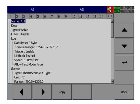
**Copy**: For example, to copy the channel configuration from channel 1 to channel 2, select the source channel, in this case Al1 (or whatever the channel is named), press on "Copy" button. Now, a "Paste" button will get enabled, go to target channel, say channel 2, and then press on "Paste" button.
