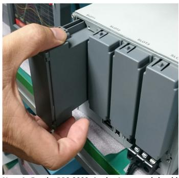
Note 4: For the PPS-3000, Analog Input card should be inserted in slots 1 to 8 only.
