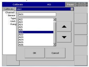
Confirm the channel to calibrate and click "Calibrate" and "yes" in the next screen
