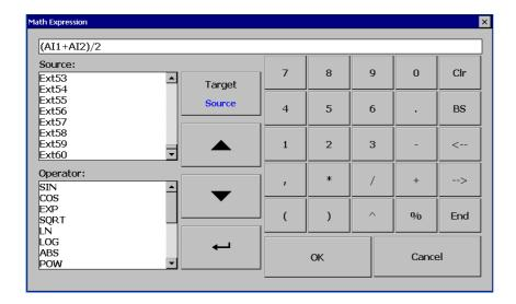
The Source covers all available Analog inputs, Digital Inputs, Math inputs, external channels.
