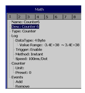
Press directional keys  $\langle \ \rangle$  at the bottom to select one of the Math channels for the Counter operation.
