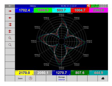
**Speed**: This is the display speed. Available options are 100 msec/dot, 1 Sec/dot, 2 Sec/dot, 5 Sec/dot, 10 Sec/dot, 20 Sec/dot, 30 Sec/dot, 1 min/dot, 5 min/dot, 10 min/Page, 30 min/Page, 1 hour/Page, 2 hour/Page, 4 hour/Page, 8 hour/Page, 12 hour/Page and 1 Day/Page.
