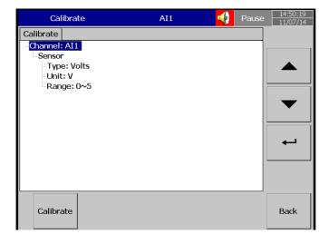
Please note that, in order to calibrate the whole Module slot accurately, the 3rd channel of each slot nust be calibrated first. Click OK.
