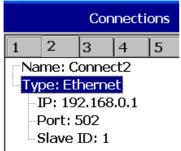
**IP:** This is enabled only if Type = Ethernet selected at any connection.
