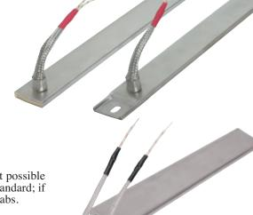
Type W2 Stainless steel braid over each lead wire offers sharp bending not possible with armor cable, as well as abrasion protection. 10" long leads standard; if longer leads are required, specify. Not available on heaters with tabs.
