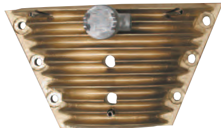
Bronze Cast-In Heater Used in Helicone Mixture to Heat High Viscosity Material
