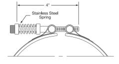
diameter heater used in the vertical position, to prevent the heater from slipping off the machine. The springs provide constant tension, therefore maintaining optimum surface contact against the cylinder being heated.
