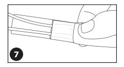
7. Press heater tape onto self-adhesive terminal flap.
