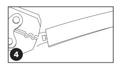
4. When using 4-wire tape in full series connection, crimp half of a #092 connector onto center two wires and trim short.
