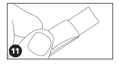
11. Use crimps to join wires.
