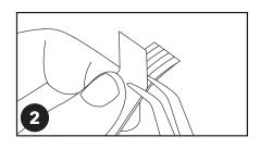
2. Split tape and open using tweezers. Dull tweezers are better than very sharp tweezers.
