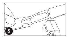
5. Crimp lead wires onto heater wires. To avoid breaking, do not crimp heater wire too hard!
