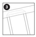
3. Apply Heat Transfer Tape across end loops and roll down firmly.
