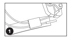
1. Push lead wires through terminal block holes. Strip lead wire ends and crimp butt connectors onto lead wires.
