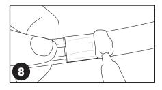
8. If desired, apply RTV Sealant over terminal block end.
