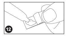
12. Apply RTV Sealant over entire end and between top & bottom lamination flaps.
