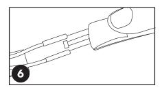
6. Strip paper liner back about 1" from tape lead end. Push terminal block over connectors.
