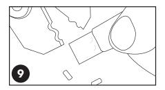
9. Split tape end open approx. 3/4" & scrape wire ends per steps 2 & 3 on previous page. DO NOT cut top & bottom tape laminations. Use half of #092 connector & crimp wire pairs together.
