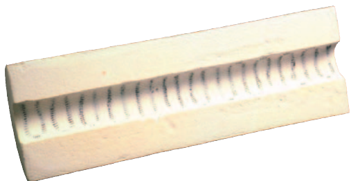
Standard Temperature (1100°C) Semi-Cylindrical Heater 2" I.D. × 6" O.D. × 18" Long 1130W, 240V
