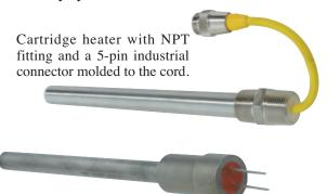
Cartridge heater for continuous air heating application with Incoloy® sheath, custom machined fitting and silicone rubber moisture barrier.
