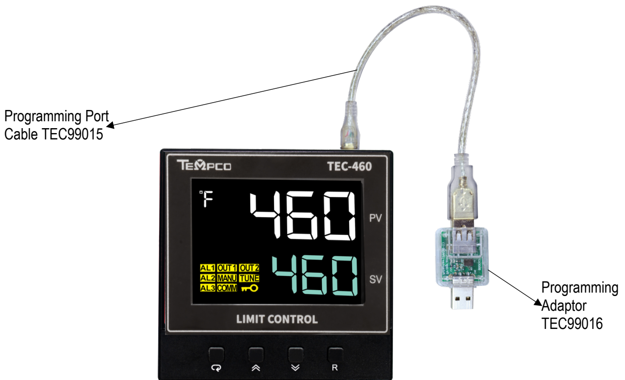
1-2 Programming Port Connection with Programming Port Adaptor
