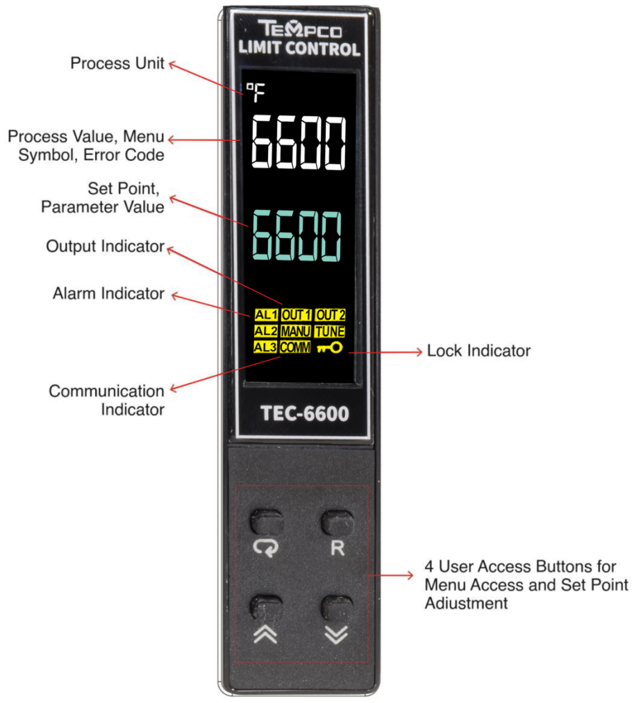
1-5 TEC-6600 Front Panel Keys and Display
