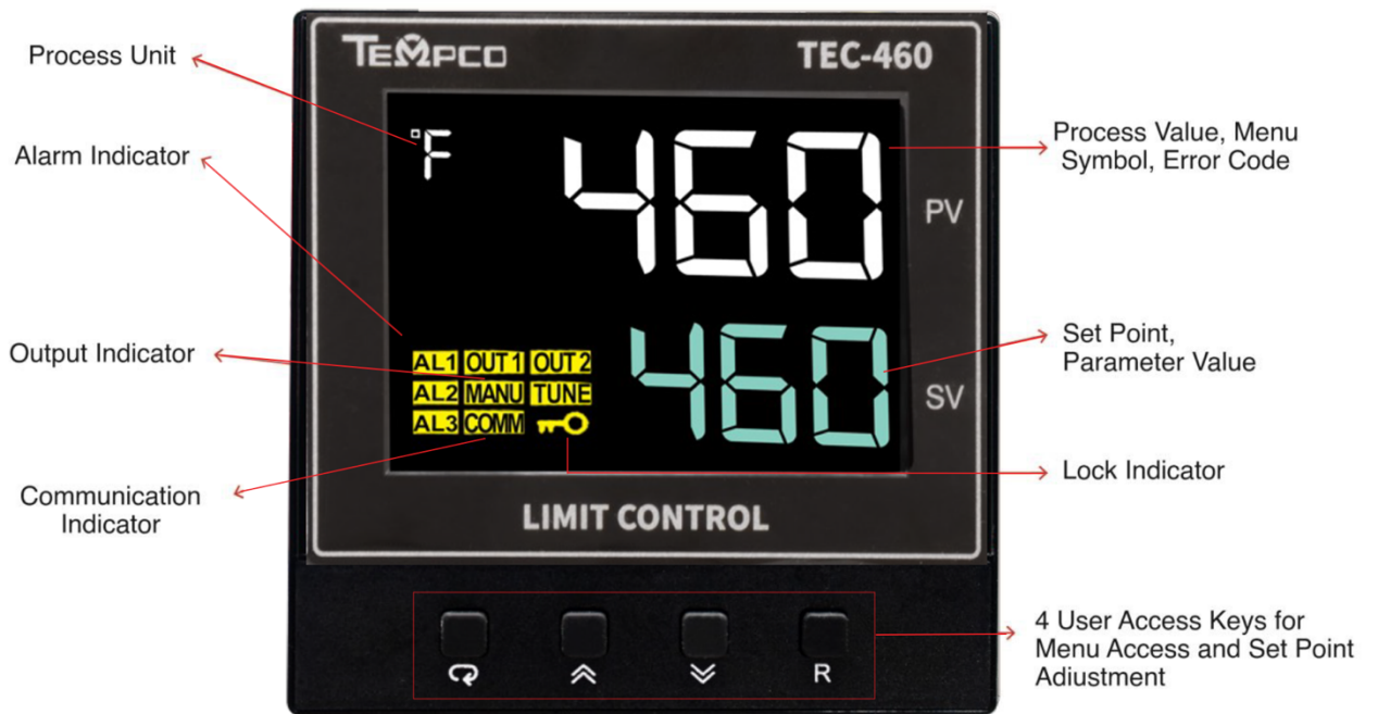
1-3 TEC-460 Front Panel Keys and Display
