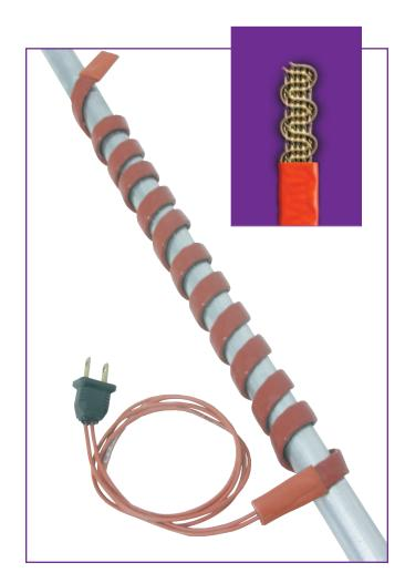
The same proven internal design of all Duo-Tapes of knitted Amox yarn over serpentined resistance is used. The heavy silicone rubber extruded outer cover provides abrasion and dielectric protection for the heating element.
