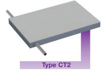
Cooling tubes exiting through the thickness opposite of each other toward the ends of the width or length.
