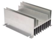
**Part Number: RLS90019 Size:** 4.75"W × 5.50"L × 2.63"H **Rating:** 0.70°C/W Pre-drilled for one or two 1-phase SSR (8-32) Panel mount 4.50" × 4.42" centers
