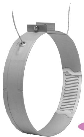
An alternative to wound ribbon core heaters is the sinuated heater element. In this type of construction, the heating element resistance wire is sinuated, or "formed" back and forth without a middle core layer of mica insulation. The heating element is then sandwiched between two layers of specially selected mica insulation to provide excellent thermal conductivity and dielectric strength.
