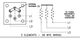
CAUTION! HEATERS DESIGNED & PRE-WIRED FOR THREE-PHASE WYE CAN NOT BE REWIRED TO SINGLE-PHASE OR THREE-PHASE DELTA WITHOUT CAUSING PREMATURE HEATER FAILURE. CONSULT TEMPCO BEFORE ATTEMPTING INTERNAL BUSSING CHANGES.
