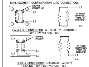
DUAL VOLTAGE HEATER NOTE: HEATERS WITH TWO ELEMENTS MAY BE USED AS DUAL VOLTAGE HEATERS. WHEN WIRED IN PARALLEL, FOR LOW
